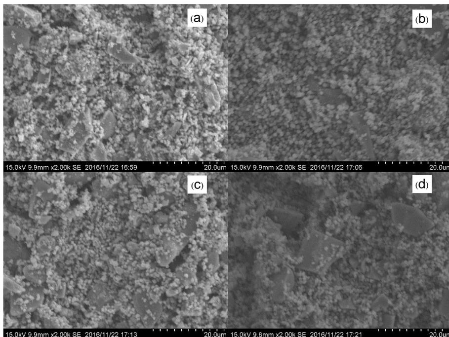
**Figure 2.** SEM images of photocatalysts sintered at different atmospheres: (a)  $\text{TiO}_2$ , (b) 1Ag- $\text{TiO}_2$  (Air), (c) 1Ag- $\text{TiO}_2$  ( $\text{N}_2$ ), and (d) 1Ag- $\text{TiO}_2$  ( $\text{H}_2$ ).
