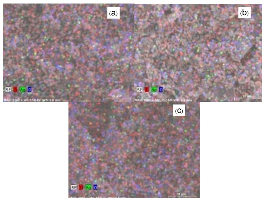
**Figure 3.** Elemental mapping of (a) 1Ag- $\text{TiO}_2$  (Air), (b) 1Ag- $\text{TiO}_2$  ( $\text{N}_2$ ), and (c) 1Ag- $\text{TiO}_2$  ( $\text{H}_2$ ).
