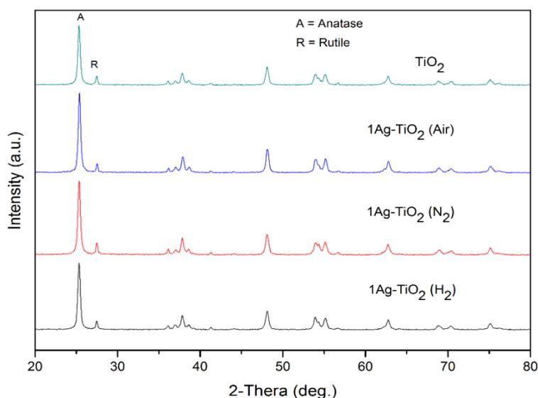
**Figure 4.** XRD patterns of synthesized  $\text{TiO}_2$  and  $\text{Ag-TiO}_2$  sintered under different atmospheres.
