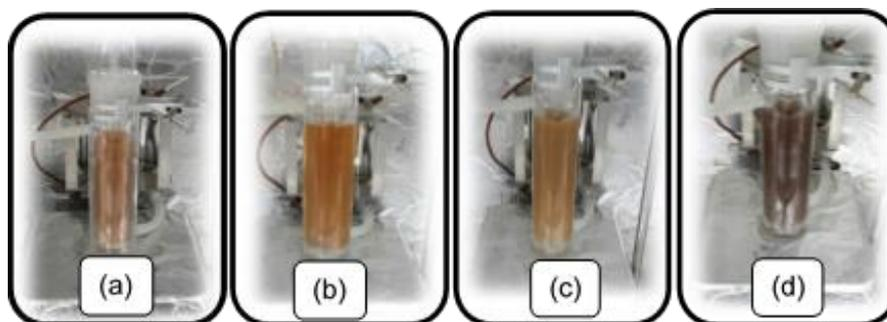
**Figure 5.** Lignin solutions before UV irradiation; (a)  $\text{TiO}_2$  (b) 1Ag- $\text{TiO}_2$  (Air) (c) 1Ag- $\text{TiO}_2$  ( $\text{N}_2$ ) (d) 1Ag- $\text{TiO}_2$  ( $\text{H}_2$ ).
